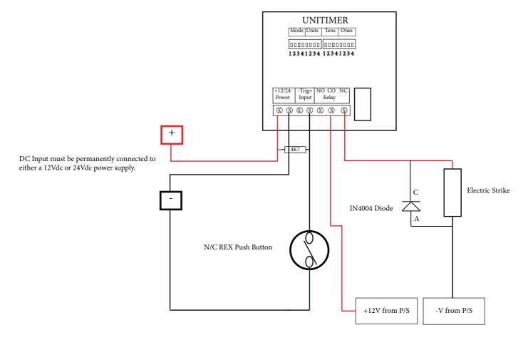
The relay can be programmed for fail safe and fail secure operation.
