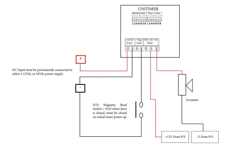
The relay can be programmed for fail safe and fail secure operation.
